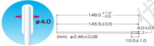
①全长: 146.0±1.0 (-0.5) mm ④棉端和轴端的距离 D≥1mm
